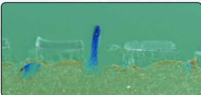
Clear Coat Defect
