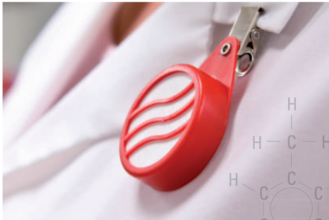
To monitor the individual exposure to toxic chemicals, the AirChek Dosimeter Badge is simply clipped onto the work clothes at a point as close as possible to the breathing zone.
